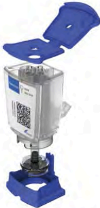
Fig. 1. Cepheid GenXpert system. (A) Instruments with 1- to 16-cartridge capacity. (B) Exploded view of GenXpert cartridge. (Courtesy of Cepheid, Sunnyvale, CA; with permission.)
