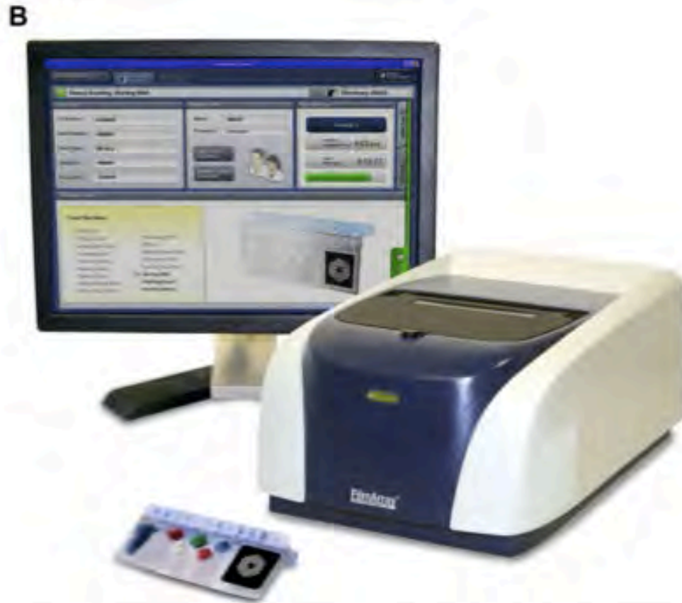
Fig. 6. BioFire FilmArray respiratory panel assay. (A) FilmArray RP Pouch. (B) FilmArray instrument and pouch. Instrument footprint in inches: 10.00 width × 6.5 height × 15.5 depth. A computer is required for operation. (Courtesy of BioFire Diagnostics Inc, Salt Lake City, UT; with permission.)
