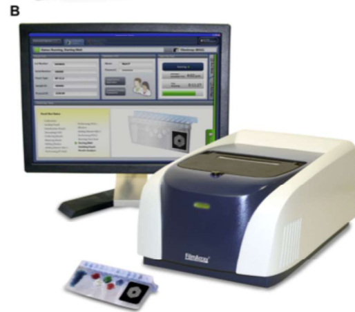
Fig. 6. BioFire FilmArray respiratory panel assay. (A) FilmArray RP Pouch. (B) FilmArray instrument and pouch. Instrument footprint in inches: 10.00 width x 6.5 height x 15.5 depth. A computer is required for operation. (Courtesy of BioFire Diagnostics Inc, Salt Lake City, UT; with permission.)
