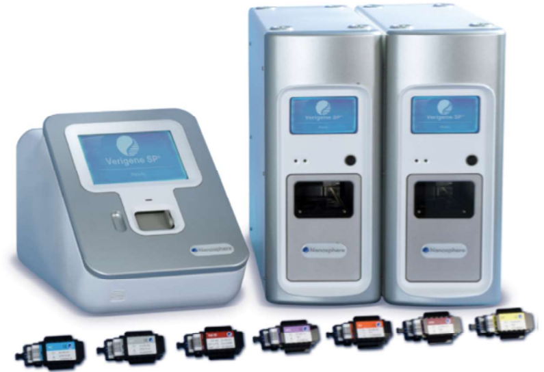
Fig. 3. Nanosphere Verigene system. Verigene processor on the right, reader and cartridges on the left. Instrument footprints in inches: Processor, 7.6 width × 18.7 height × 22.9 depth; reader, 11.7 width × 12.4 height × 20.5 depth. Processors are stackable. No computer is required for operation. (Courtesy of Nanosphere, Northbrook, IL; with permission.)
